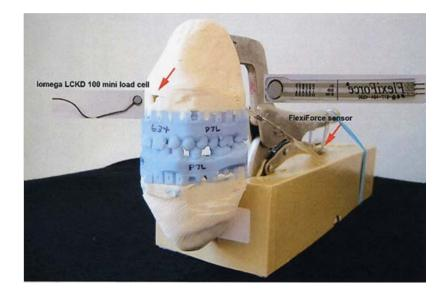
Figure 14. Illustrate a completely assembled pattern replication device with a channel
