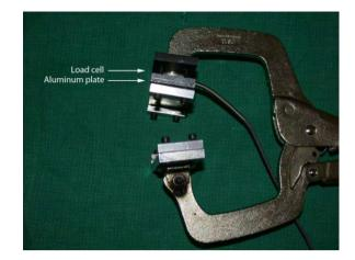
**Fig. 1.** The improved biting device consisted of a vice grip with an aluminum plate fixed to the upper anvil. This aluminum plate receives the pressure of the dentition during the biting action and transfers it to a load cell that is connected to a calibrated digital readout.
